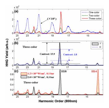
FIG. 3 (color online). (a) Comparison of the maximum harmonic yields driven by different laser fields. (b) Comparison of the harmonic yields driven by the three-color laser field with two different relative phases. (c) Comparison of the harmonic yields driven by the three-color laser field with different intensity and density conditions.
