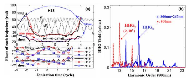
FIG. 4 (color online). (a) The phase of the 18th harmonic in different laser fields (upper panel) and the comparison with the adjacent 16th and 17th harmonics (lower panel). (b) The harmonic spectra in two polarization directions (HHG<sub>v</sub>, HHG<sub>v</sub>).
