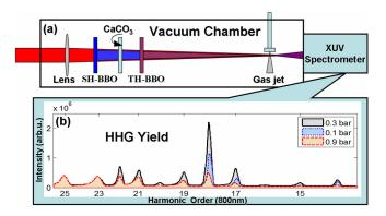
FIG. 1 (color online). (a) Schematic of the experimental setup. (b) Harmonic spectra obtained with different gas pressures.
