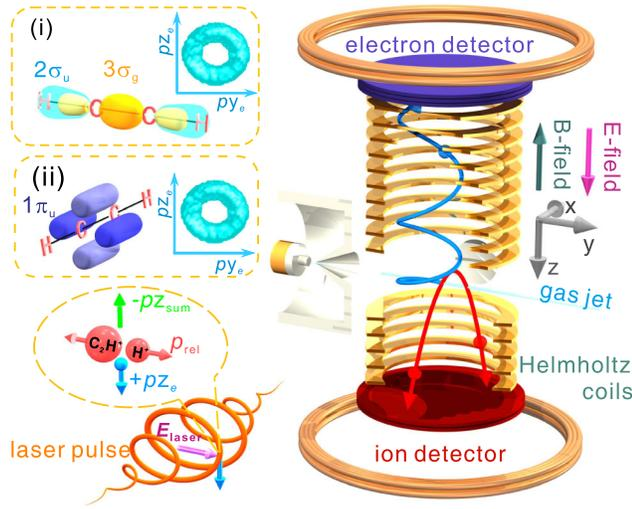
FIG. 1 (color online). Schematic diagram of the experimental apparatus. The insets schematically illustrate that (i) both the molecular axis of the acetylene and the freed electrons (blue donut) lie in the polarization plane for the dominance of the  $\sigma$  orbitals, whereas (ii) the acetylene is oriented perpendicular to the polarization plane for the dominance of the  $\pi$  orbital.
